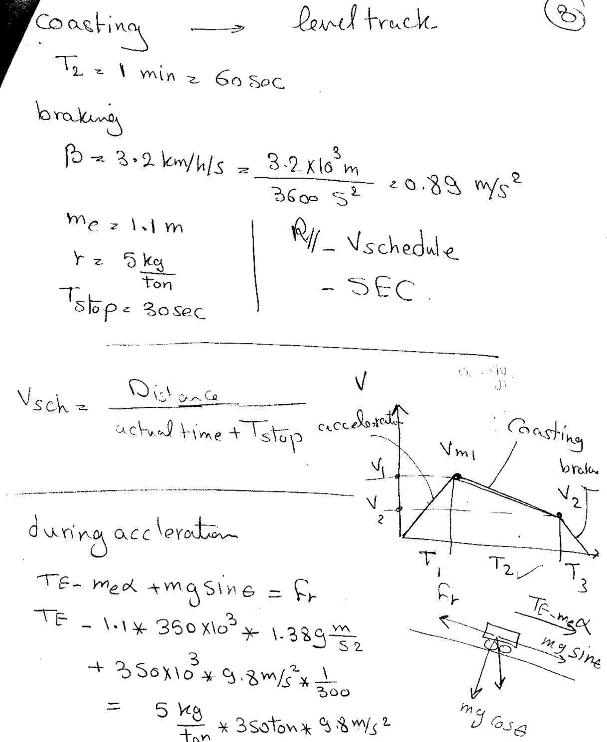
$\frac{5 \log}{T_{nn}} \times 3 \text{ soton} \times 9.8 \text{ m/s}^2$ TEI = 535231.67 W
