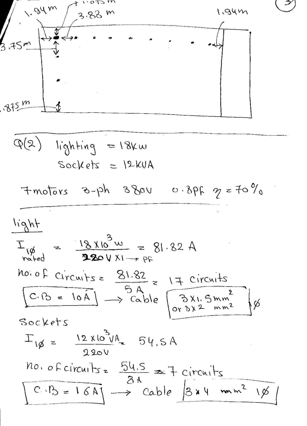
5×4mm2 30 motor Shp Irated z 10.12A/ph Ist > 40.48A ~ CB = 50A cable > 29.3A -> Calle = 5 × 2.5 mm<sup>2</sup> ЗØ
