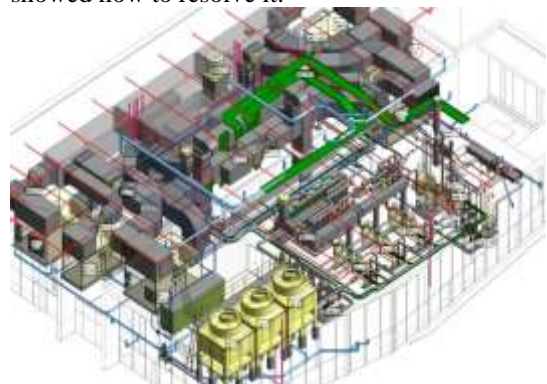
Fig. 14- Hospital BIM modeling-MEP
