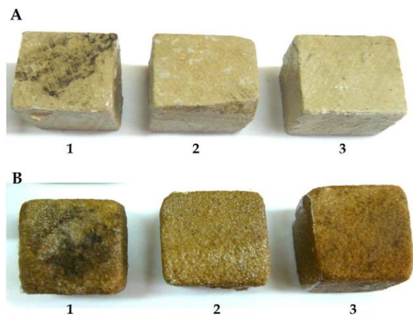
Fig. 3. The antifungal activity of the acrylic polymer and silicon polymer loaded with nanosilver structures (40 mg/ml) against Aspergillus flavus : (A) represents limestone blocks treated with functionalized silicon polymer (2) and functionalized acrylic polymer (3) while (B) represents the sandstone blocks treated with functionalized silicon polymer (2) and functionalized acrylic polymer (3). Stone blocks number 1 in both (A) and (B) represent the untreated stones.
