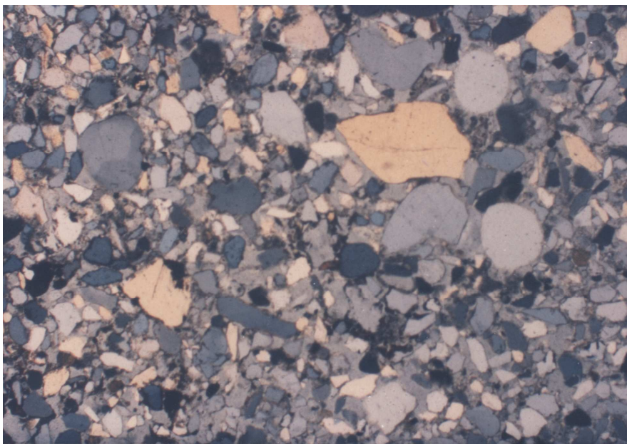
Figure (6) Skel ferriargillans. Thin section under crossed polarizers, 80X.
