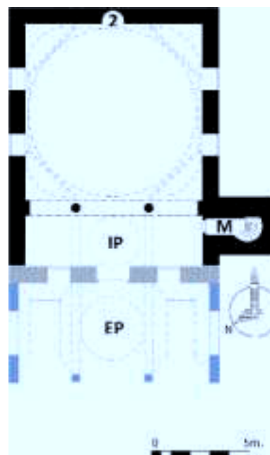
30. Plan of Fethiye mosque of Nafpaktos; a presumptive reconstruction with an addition of an inner portico in front of the prayer hall including the minaret's door plus an external portico "Riwaq" (May 2008)
