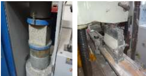
Fig. 4. Compressive Strength Testing of Concrete cube and indirect-Tension Test for Concrete Cylinder
