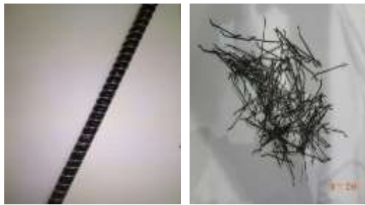
Fig. 2. BFRP bar and steel fibers used for Beam Reinforcement
