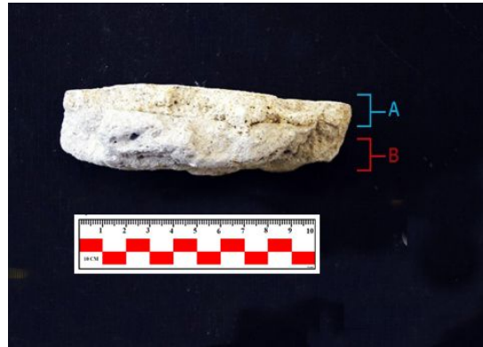
Fig.7 Two layers of the flooring mortar sample WM8
