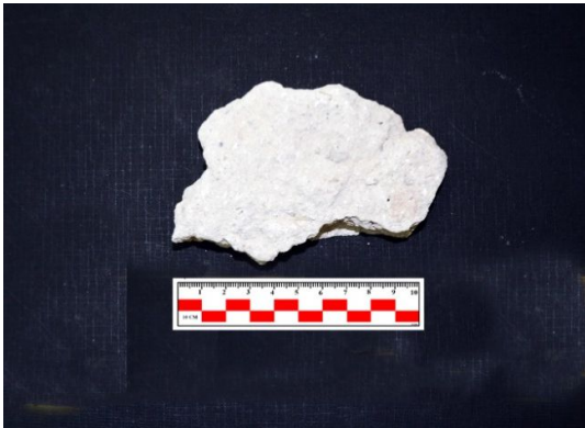
Fig.6 Flooring mortar sample WM1
