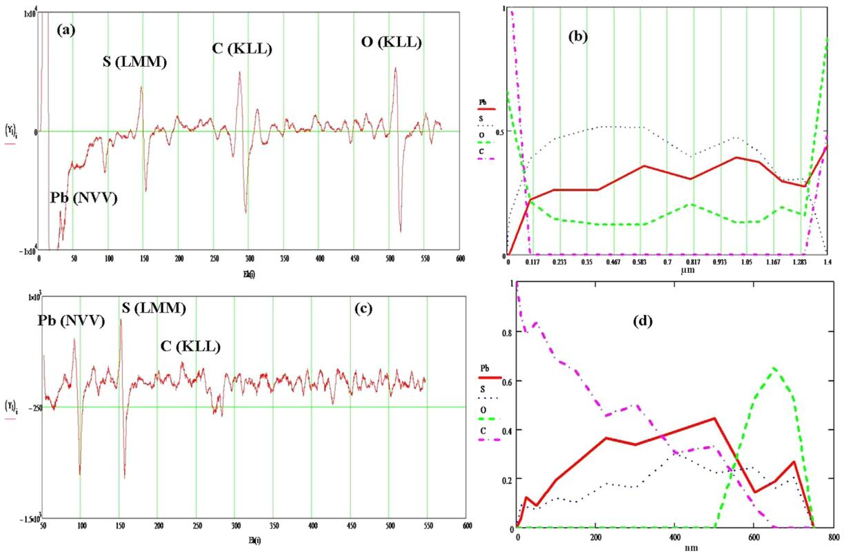
**Fig. 5.** AES spectra of photosensitive PbS films. (a) corresponds to Auger spectrum from samples produced by PVD, (b) shows the ratio of elemental structure to depth of samples prepared by PVD, (c) corresponds to Auger spectrum from samples produced by CVD, and (d) shows the ratio of elemental structure to depth of samples prepared by CVD.
