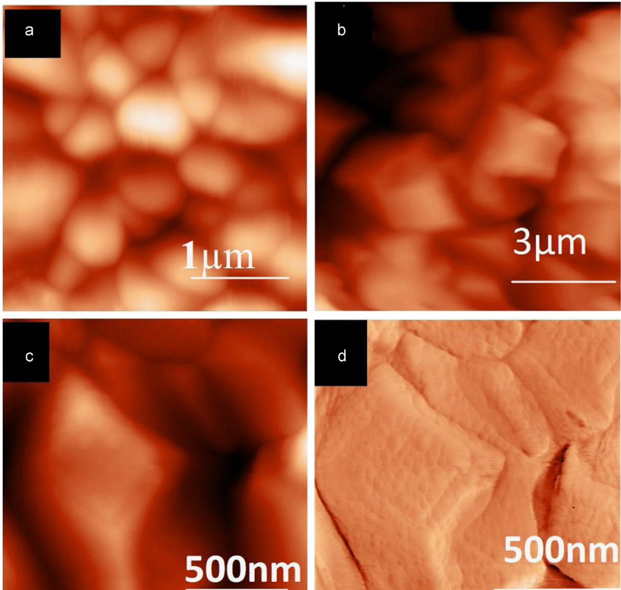
**Fig. 2.** AFM picture of photosensitive PbS films. (a) corresponds to scan the surface of the photosensitive layer produced by CVD, (b) corresponds to scan the surface of the photosensitive layer produced by PVD, (c) scan the PVD films in nanoscale to obtain the small grains in each cubic and (d) signal LF for PVD.
