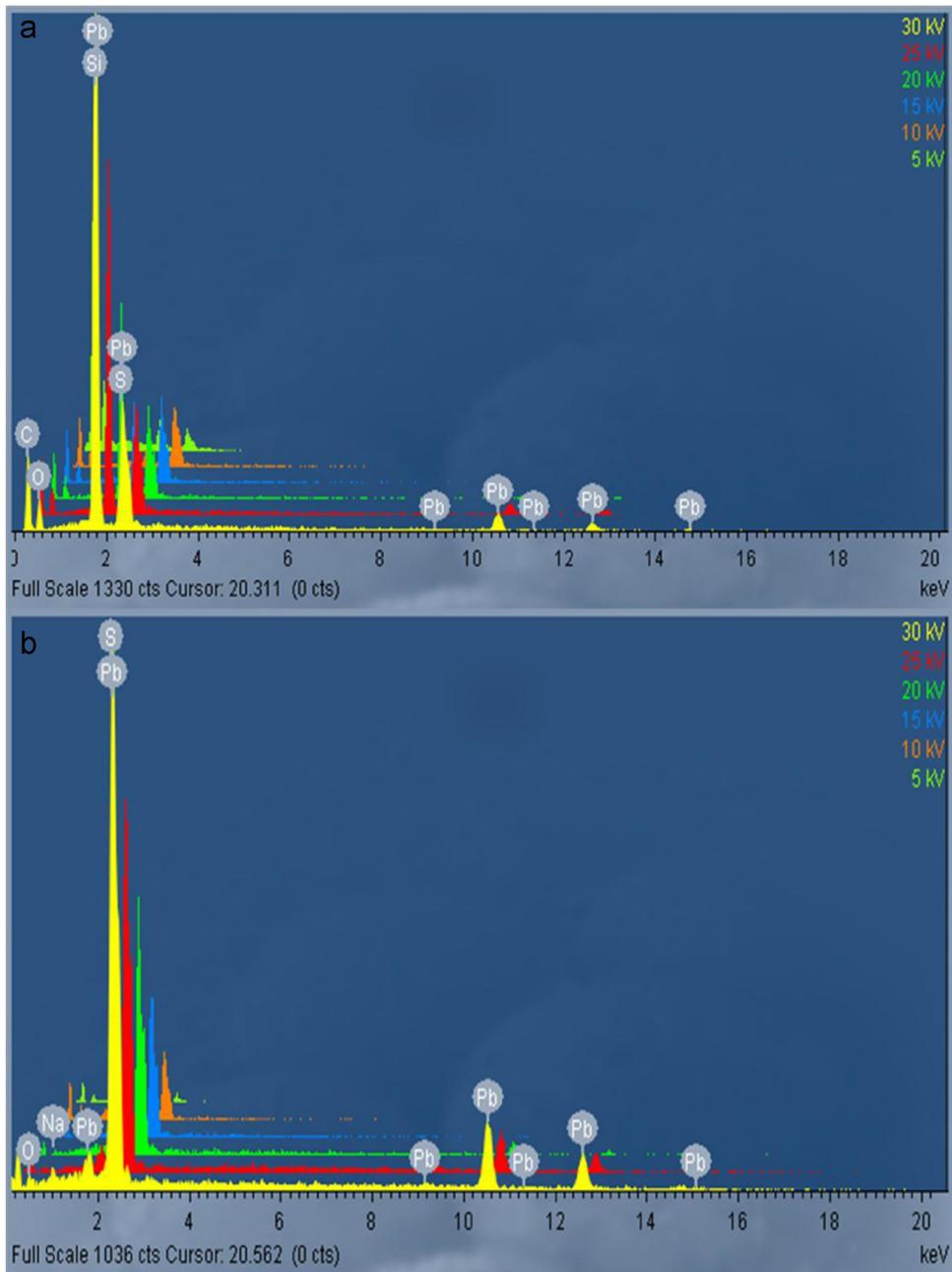
Fig. 4. EDXS spectra of photosensitive PbS films. (a) Films prepared by CVD and (b) films prepared by PVD.
