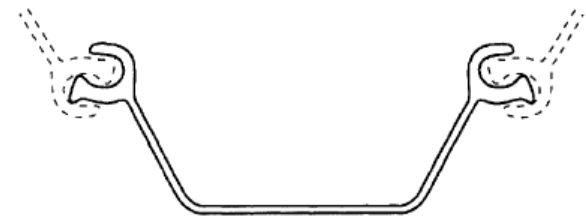
(c) Arch-web piling
